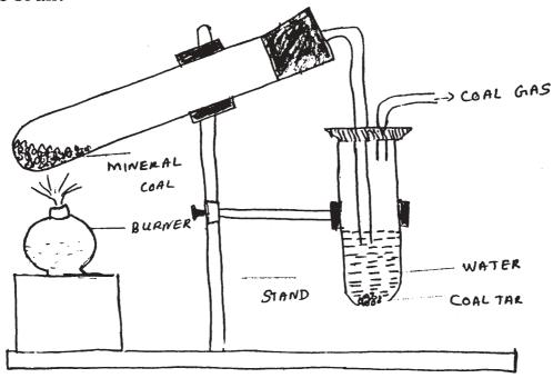
Observation: The gas which come out from the end of the tube is coal gas. It burns with blue flame.
